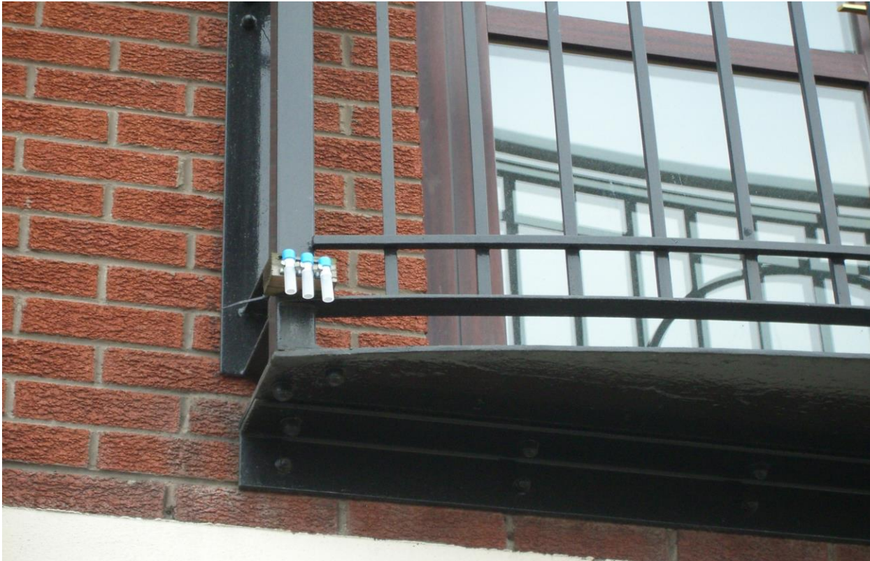
Figure 7. Picture of triplicate diffusion tubes on façade of Normandy Court
